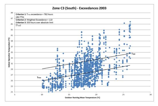
Based on the recommendations of TM52 each of the representative zones from all three buildings are shown to have a risk of overheating when operating in free running mode for the 2003 DSY.
