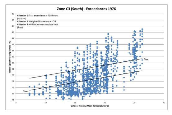
Based on the recommendations of TM52 each of the representative zones from all three buildings are shown to have a risk of overheating when operating in free running mode for the 1976 DSY.
